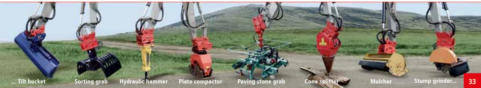
... Tilt bucket    Sorting grab    Hydraulic hammer    Plate compactor    Paving stone grab    Cone splitter    Mulcher    Stump grinder...
